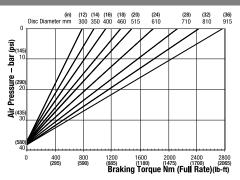
Minimum Pressure for full retraction: 50 bar (725 psi) Maximum Braking Force full rate: 6.4kN (1438.77 lbf) Weight of caliper and thruster - 11kg (24.25 lb) Weight of thruster only - 4.0kg (8.81 lb) Volume displacement of thruster at 4mm (0.16 in) retraction = 5ml (0.16 fl oz)
