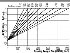
Minimum Pressure for full retraction: 6.4 har (93 psi) Maximum Braking Force XS 9.6: 14.3kN (3214.76 lbf) Weight of caliper and thruster - 12.1kg (26.67 lb)
