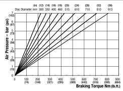
Maximum Pressure 7 bar (102 psi) Maximum Braking Force = 1.9kN @ 7 bar (427.13 lbf @ 102 psi)
