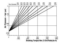
Minimum Pressure for full retraction: 17 bar (247 psi) Maximum Braking Force 1/3rd rate: 2.2kN (497.57 lbf) Weight of caliper and thruster - 11kg (24.25 lb) Weight of thruster only - 4.0kg (8.81 lb) Volume displacement of thruster at 4mm (0.16 in) retraction = 5ml (0.16 fl oz)
