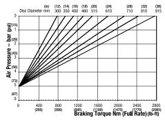
Minimum Pressure for full retraction: 5 bar (73 psi) Maximum Braking Force full rate: 6.4kN (1438.77 lbf) Weight of caliper and thruster - 10.5kg (23.14 lb) Weight of thruster only - 3.5kg (7.71 lb) Volume displacement of thruster at full retraction = 950ml (32.12 oz)
