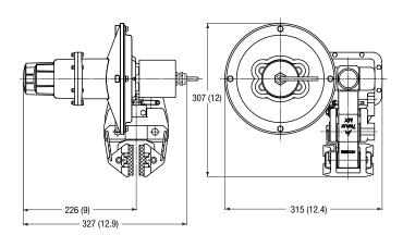
Maximum Braking Force = 6kN (4425 ft lb) Weight of caliper and actuator - 15.7kg (34.61 lb) Weight actuator only - 8.7kg (19.18 lb) Weight of controller - 5.5kg (12.13 lb) The EA actuator is a spring applied, electrically released unit designed for use with the Twiflex MX range of disc brake calipers. A 175W pancake motor drives a ball screw mechanism, retracting the brake.
