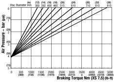
Minimum Pressure for full retraction: 5.5 bar (80 psi) Maximum Braking Force XS 7.5: 11.2kN (517.86 lbf) Weight of caliper and thruster - 11.9kg (26.23 lb)
