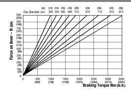
Weight of caliper and lever assembly - 8.4kg (18.51 lb) Weight of lever assembly only - 1.4kg (3.08 lb) Maximum Braking Force = 8.3kN @ 0.9kN force on lever (1865.91 @ 202.32 lbf force on lever)
